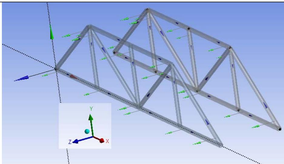
When there are two parallel lattice beams, the points on the lower base will be joined.
