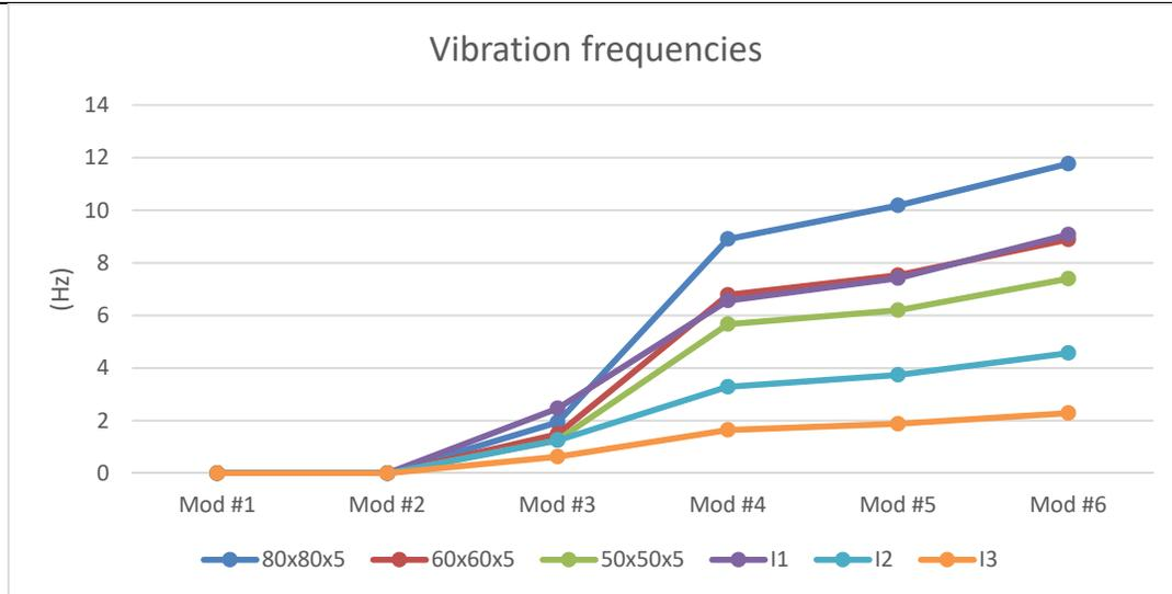
For equivalent profiles in terms of the value of the section surfaces, it can be seen that the rectangular profile generates its own vibrations with higher frequencies than the I profile.
