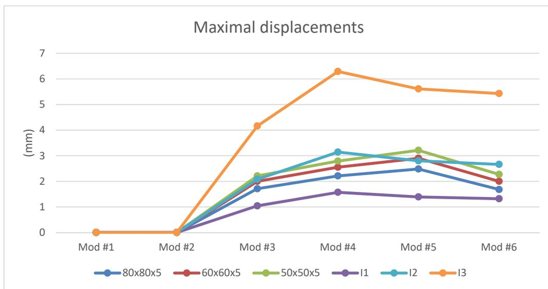
From the point of view of the total displacements, it is observed that the maximum values are found in the own vibration modes Mode # 4 or Mode # 5, after which they decrease with the increase of the own vibration frequencies.
