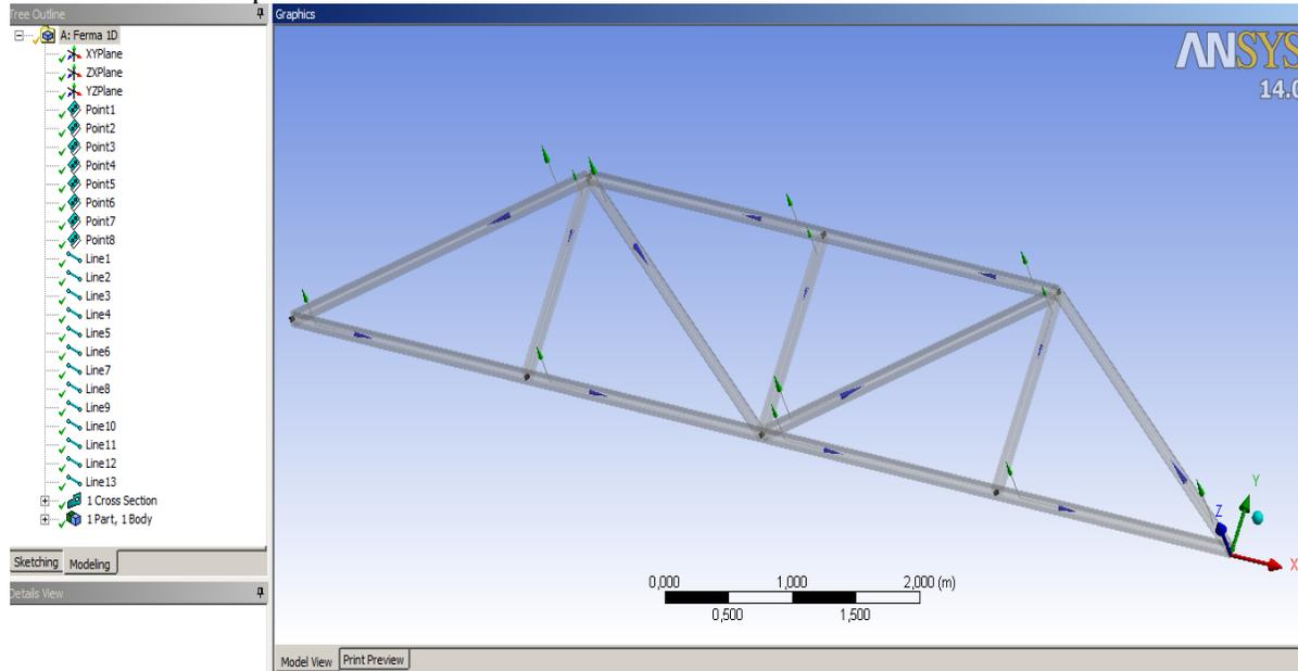
The geometry of the bridge can be continued in two ways: either by building a number of 8 points corresponding to the beam in a plane parallel to the one in which the original model was built (at  $z = 1.5$  m) or by copying the existing beam at distance of 1.5 m on the  $Oz$  axis.
