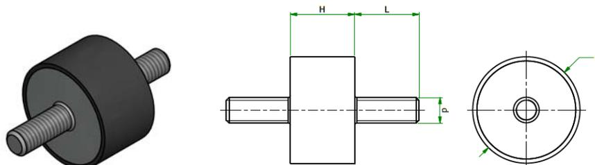
These elements are frequently introduced in the subsystems of motor vehicles having the role of supporting parts or as elastic quasi-couplings with damping, bringing the following advantages: they eliminate wear and
